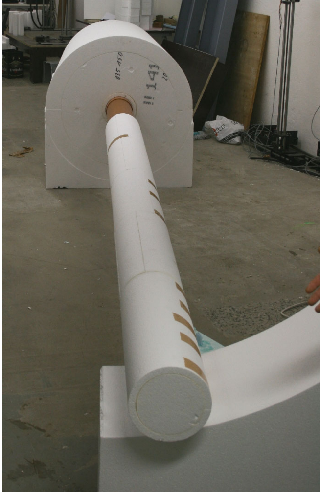
Pin needle out of pvc hose, EPS covered
